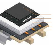
APOLLO OST MOGAFIX KSK-U DR MOGADÄMM (MIFA / PUR / EPS / PET) MOGAT SDF 18 MOGAFIX KSK-D Uni Beton, Trapezblech, Holz
